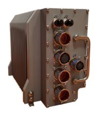
HydeDM™ 302 is a Form / Fit / Function+ replacement for the IDM 302 that requires no changes to aircraft wiring or Operational Flight Programs (OFPs) and makes the F-16 immediately interoperable with US and allied forces using Joint CAS (JCAS) digital messaging standards for Digitally-Aided CAS (DACAS).
