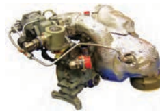
Emergency Power Unit
